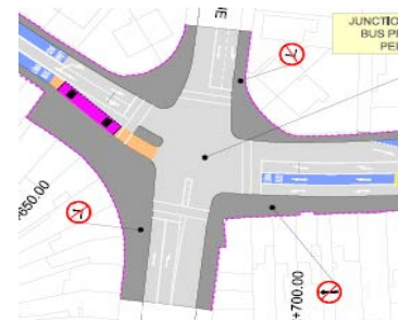
Figure 27 Bus stop located very close to the junction
