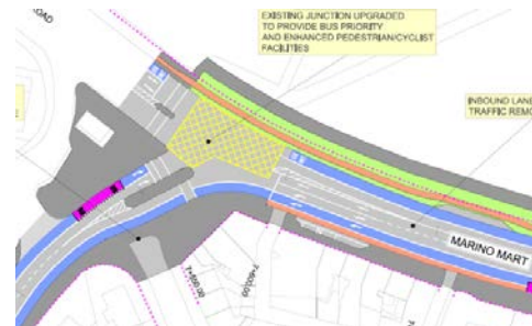
Figure 14 Cycleway abruptly stopping on Marino Mart
