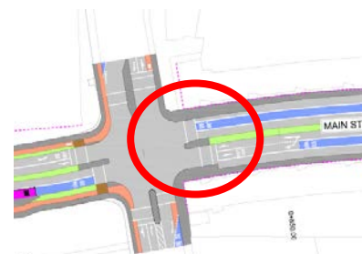
Figure 4 Example of lack of cycle facilities at a major junction
