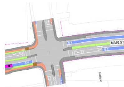
Figure 3 Example of bus lane abruptly beginning
