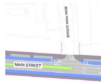
Figure 1 Example of Bus lane with no alternative cycle facilities
